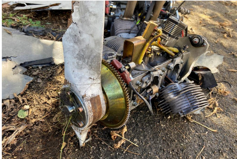
Engine of a destroyed Shahed-136 / Open-source photo
